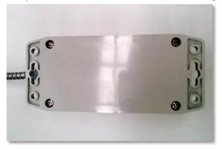
4. Remove the four module screws. Carefully open the module.
