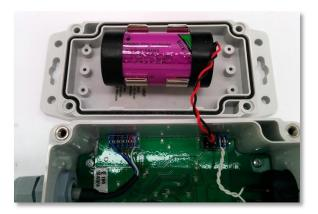
10. Close the module by lifting and then turning the printed circuit board portion of the module on top of the battery portion of the module. This will avoid the insulation Oring from falling out of its groove.
